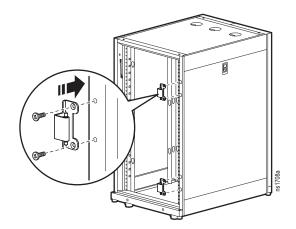
7. Remove screws securing the hinges in the door frame.
